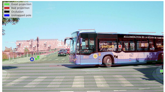
Fig. 3: Projection of map features onto an image frame using Patchwork++.
