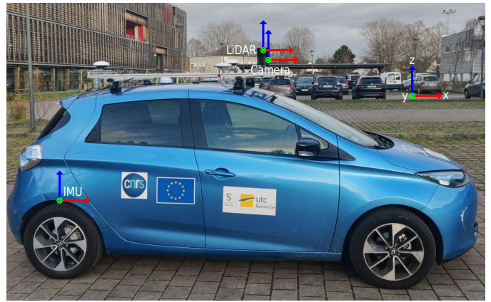
Fig. 6: Experimental Renault ZOE vehicle equipped with a NovAtel SPAN-CPT GNSS/IMU and a Hesai Pandora sensor.
